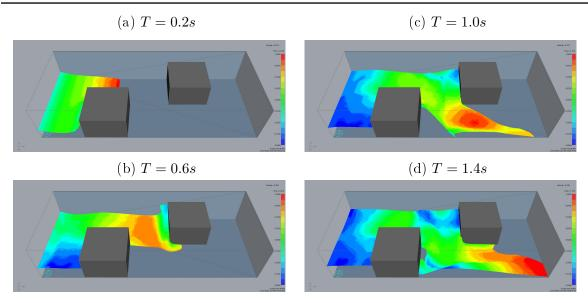
Figure 14: Iso-surface of SURN = 0.5 coloured by velocity magnitude
