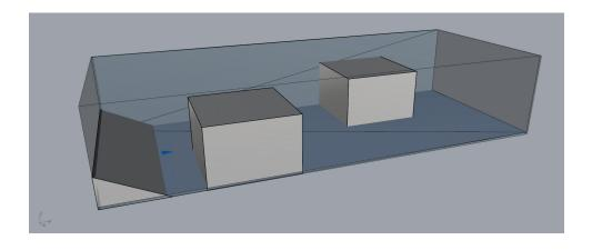
Figure 1: Simulation set up with two obstacles in the channel. The wedge is used only at the start of the simulation to initialise the inflow of water from left to right.
