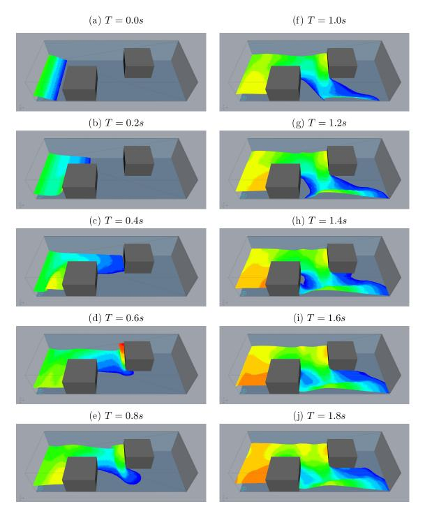
Figure 15: Iso-surfaces of SURN = 0.5 coloured by the water height above the floor
