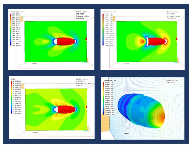
A spherical indented base was added, and the calculated mass of the bullet matched Eley data to about 2% (assuming a bullet-density of Lead). The calculated Cd at this speed, with no angle of incidence, was 0.564 based on.22 inch diameter and 1000 fps [= 304.8 m/s]. It might be expected that when modelled "at incidence", the drag will increase slightly (perhaps 20% at a few degrees).
