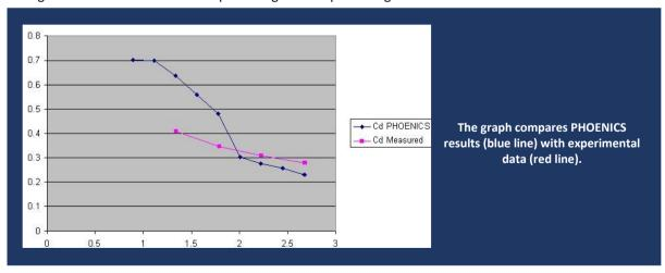
Experiments show a slightly higher drag coefficient which may be due to the bullet actually flying at a small incidence as it 'cones' around its direction of flight.
