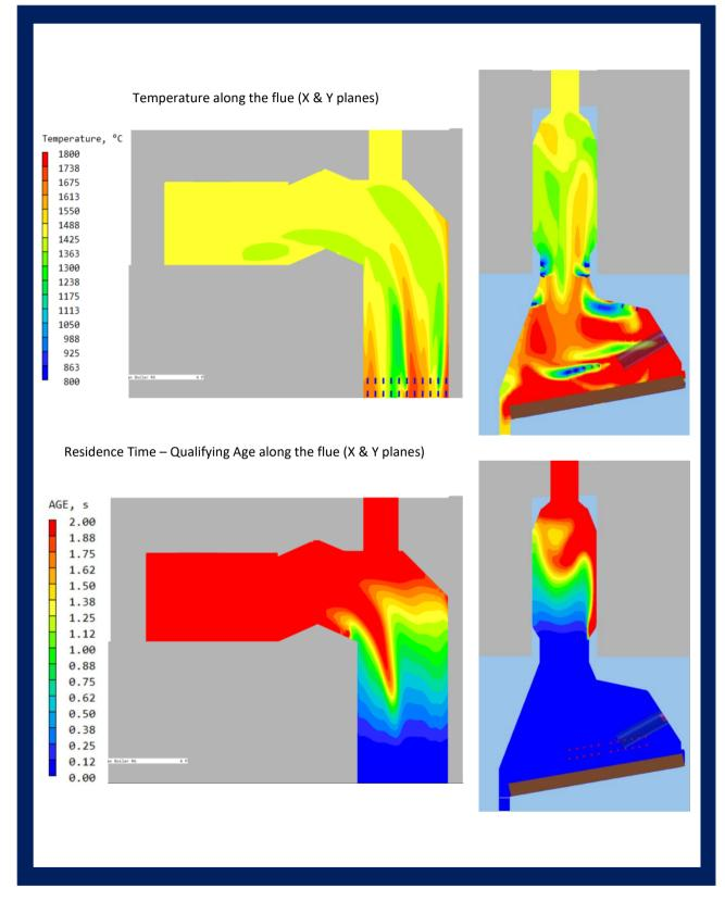
The CFD results indicated that the minimum gas temperature throughout the qualifying zone met or exceeded the target values. Similarly, the results confirmed that operational testing of the proposed design of the combustion chamber was likely to meet or exceed the residence time and temperature targets recommended in the Incineration of Waste Sector Guidance Note EPR 5.01.
