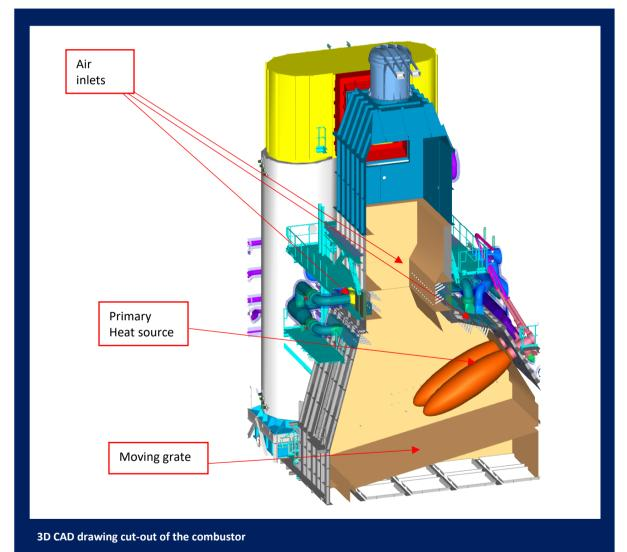
The entire volume of the combustor is embodied in the CFD model, including each individual recirculation inlet. The upper section of the combustor is also modelled, corresponding approximately to the section shown in yellow (above.)
