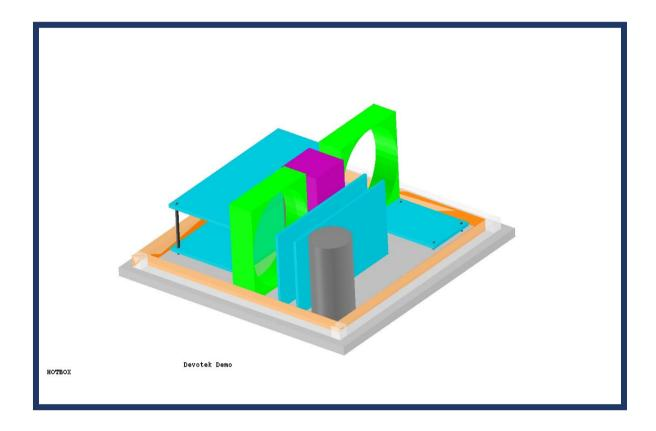
A relatively coarse mesh of 119 x 141 x 76 was applied. Given the nature of the geometric features, PARSOL, was not required. The IMMERSOL radiation model was activated, with the LVEL turbulence model selected, and a transient (time-dependent) operation of 10 time steps covering a 5-minute period. The run time, on a 3GHz PC was 12.7 hours.
