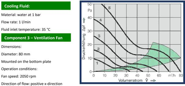
Pressure raise ("Druckerhöhung") as function of the volume flow rate ("Volumenstrom") as depicted for line 2.
