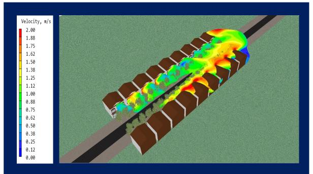
Figure 7: Iso-surface plot of temperature at 19 °C, coloured by velocity, demonstrating that the majority of the street experiences at least 1 °C of cooling due to evapotranspiration.
