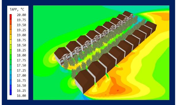
Figure 6: Contour plot of apparent temperature at pedestrian level showing up to 3 °C of cooling towards the leeward end of the street. Scale: Red – 20 °C; Blue – 16 °C
