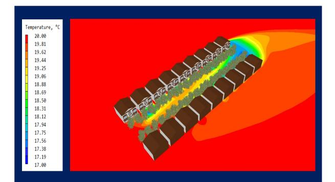
Figure 5: Contour plot of temperature at pedestrian level showing up to 3 °C of cooling towards the leeward end of the street. Scale: Red – 20 °C; Blue – 17 °C
