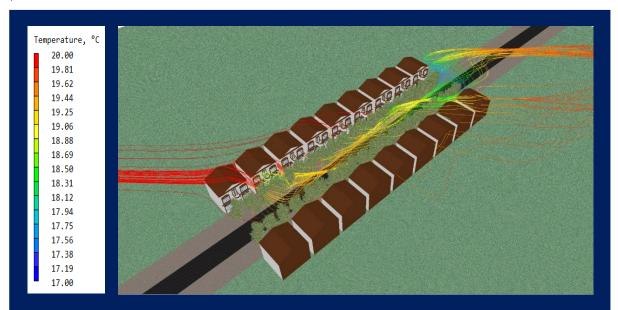
Figure 3: Streamline plot, coloured by temperature, showing the origin and destination of flow along the centre of the street at pedestrian level. Scale: Red -20 °C; Blue -17 °C
