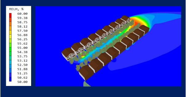
Figure 4: Contour plot of relative humidity at pedestrian level showing up to an increase of 10% humidity towards the leeward end of the street. Scale: Red – 60 %; Blue – 50 %
