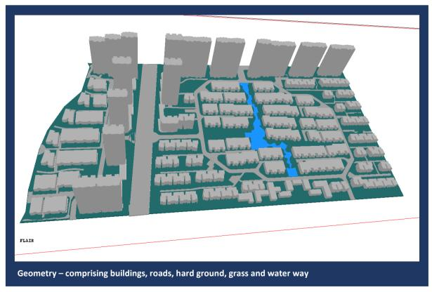
The idealised geometry shown above contains many of the components of interest to the "Heatisle" engineer; viz, concrete and glass high rise buildings, tarmac roadways, hard terrain and vegetation, and a water course. Each component responds differently to solar radiation.
