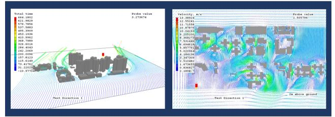
Images were generated of various views of the velocity fields at 2, 20, 40, 60, 80 and 100m above the ground; two of these are shown below.
