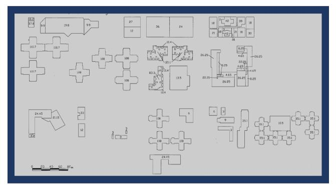
The drawing was scanned, and used as a backdrop in the AC3D software, supplied as a utility in PHOENICS/FLAIR .The outlines of the buildings were traced to create polygons, which were extruded to produce individual buildings.
