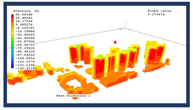
The inbuilt wind-profiling feature of PHOENICS/FLAIR was used within the model to represent more-accurately a real situation though, for this particular demonstration scenario, no representation was made of the surrounding hilly terrain which would greatly affect results.
