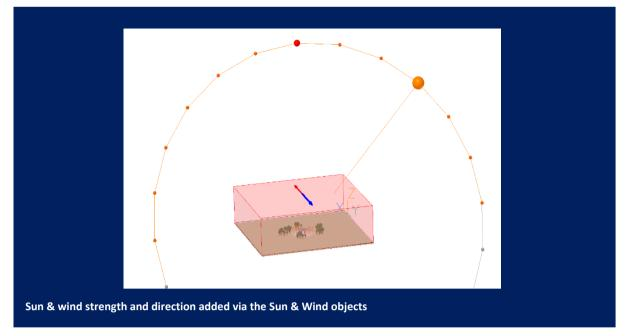
The capability of PHOENICS/Flair to interface with third party software products (such as EnergyPlus<sup>™</sup>) to extract the meteorological data for a specific location was not used on this occasion, and such data was added manually via the GUI.
