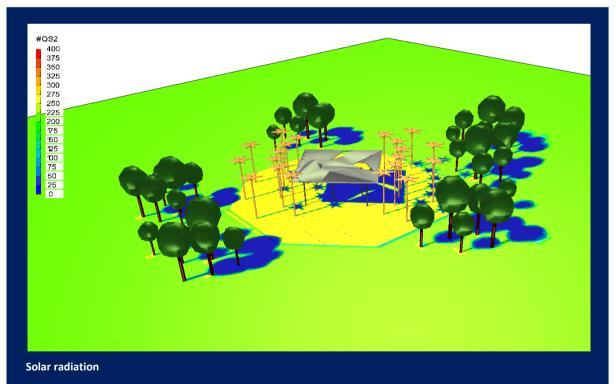
In order to make a true comparison of the results of the simulation with measured data, it is usual to run the CFD model transiently to capture the heating and cooling processes over time. For the purpose of canopy design however, this case can be run as a steady-state simulation to represent the meteorological effects taken as a snapshot in time, employing a 'solar absorption' factor to ascertain a reasonable trend.
