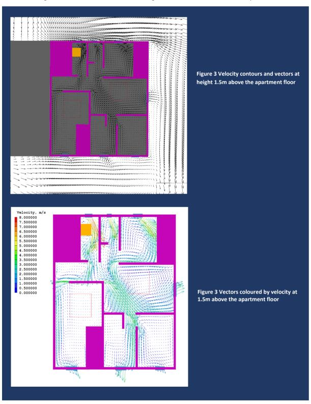
**Figure 3 shows vectors inside the apartment, coloured by velocity**. Again, we see that the flow enters the apartment through the north windows and exits at the east and south windows highlighting several regions of re-circulating air.
