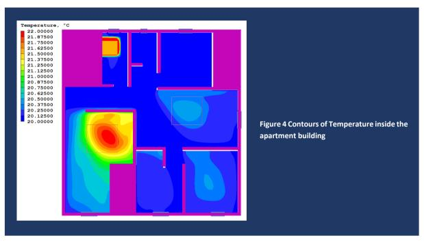
**Error! Reference source not found.** shows the temperature distribution at 1.5*m* above floor level inside the apartment. The warmer areas are where there is a combination of proximity to heat source and lack of flow movement. When warmer air inside the apartment is recirculated, we see higher temperature areas.
