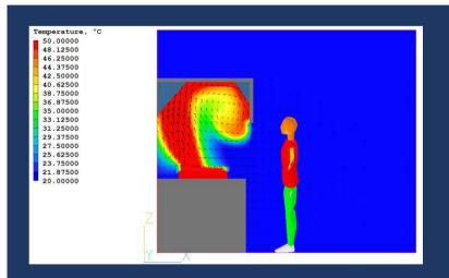
Figure 8: Temperature contours and overlaid velocity field across the whole kitchen in the case with the exhaust extraction rate reduced by 28% with the inlet jets switched on.
