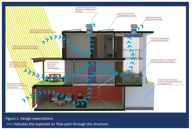
In this demonstration, PHOENICS/FLAIR is used to analyse the natural ventilation of a concept home, comparing it to initial expectations. The building is a private house, to which full recycling and bioclimatic concepts have been applied. The building consists of re-cycled shipping containers and was designed by ASOLBA Enginyeria & Arquitectura, a firm of sustainable design and energy efficiency engineers located in Guayaquil, Ecuador and Barcelona, Spain.
