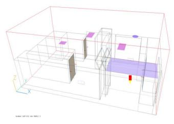
A 3D CFD model was built from 2D CAD plan drawings, provided by the client. The dimensions of the domain containing the LAF unit cleanroom were ~11.5m x 7m x 5m. Figure 1 shows a perspective view and a plan view of the room. Walls, floor and ceilings that obstruct the view have been hidden.
