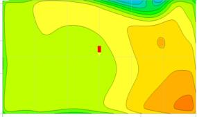
Figure 3 – Zoomed view of velocity at workbench directly beneath LAF unit
