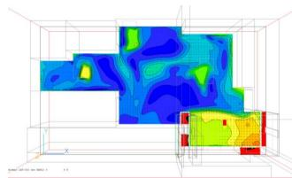
The yellow and orange region in the bottom right is the dominant flow feature of the room and represents the sinking air beneath the LAF. The red regions around it represent the high velocity air in the return ducts leading to the plenum chamber. The yellow and green regions inside the room represent flow from the three ceiling supplies towards the ground, and flow induced by the supplies and LAF.
