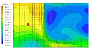
Figure 4 – Side On view showing velocity on a section across the middle of the LAF unit
