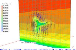
Figure 3. Velocity magnitude contour plot in the plane of a modelled turbine with superimposed in-plane velocity vectors.
