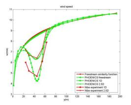
Figure 4. Comparison of PHOENICS results for the axial wind velocity with experimental results from the Nibe wind turbine experiments. The surface roughness is assumed to be 0.08m and the friction velocity 0.56m/s.
