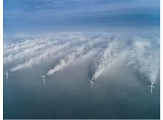
Figure 2. Horns Rev 1 is an 80 turbine wind farm off the western coast of Denmark, commissioned in 2002, and delivering 160MW. The above photograph shows the turbulence field downstream of the wind turbines. Unique meteorological conditions on 12 February 2008 at 1300 hours resulted in the wind turbines creating condensation (i.e. clouds) of the very humid air, thus making it possible to see the turbulence pattern behind the wind turbines.
