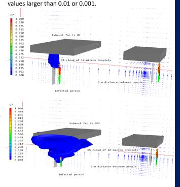
Fig. 1 Spread of cloud of 10-micron droplets with and without ventilation
