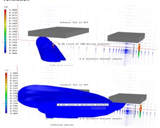
Fig.3 Spread of 0.1% clouds of 100-micron and 10-micron droplets without ventilation
