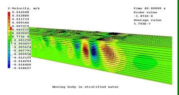
Figure 4. Surface vertical velocity contours and velocity vectors after 40s for the case starting at 60% thrust, increasing to 100% thrust after 15s.
