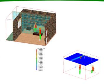
3 – PHOENICS-Flair: geometrical model and simulation of the air circulation velocity
