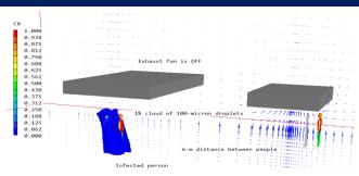
Fig.2 Spread of cloud of 100-micron droplets with and without ventilation
