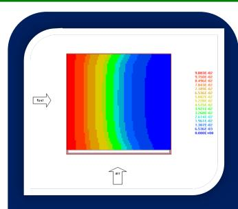
Figure 1. An early calculation with PHOENICS<sup>1</sup> for the local hydrogen distribution in a solid oxide fuel cell. 1.8s.
