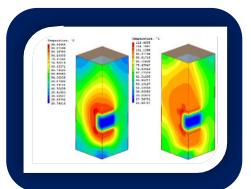
The following figure demonstrates distribution of concentration of droplets, which are formed due to condensation in the same time moments.
