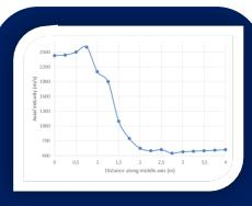
b) Axial centerline velocity of jet exhaust
