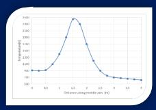
c) Axial temperature starting from jet exhaust
