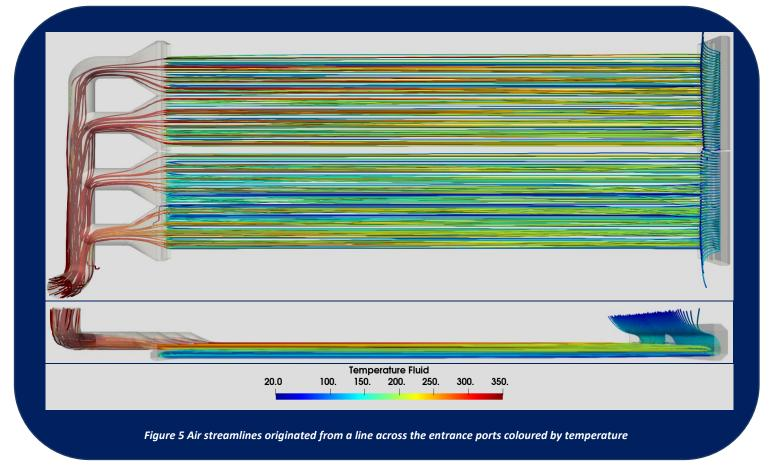
As can be seen, the source of the streamlines is chosen at above the entrance ports. Since the radiation effect has regressed, the medium entering the system is nearly at the ambient temperature.
