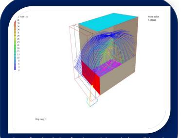
Part of a simulation for determining wind conditions in a large enclosure where work is being carried out.
