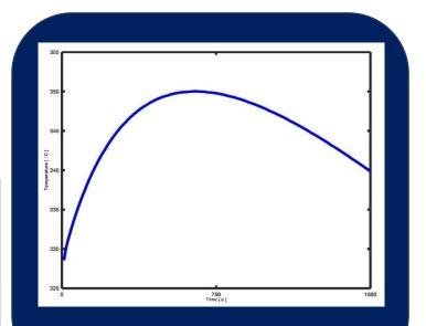
Figure 4 Temperature of the final product (air)
