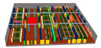
The predicted power output from any chilling device can be determined and is useful for highlighting which units are not providing sufficient cooling, and which are only partially loaded. Results might indicate a re-distribution of the units to optimise the cooling, or even fewer units required thus providing cost savings.
