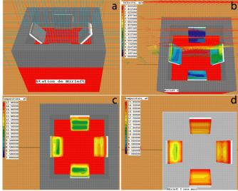
Mesh, velocity and temperature contours on the four condensers
