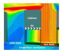
Results from the simulations show the air flows and temperatures into and out of the cabinets, indicating undesirable regions of recirculation from hot to cold aisles. PHOENICS also enables average and maximum inlet and outlet temperatures to all cabinets to be evaluated.
