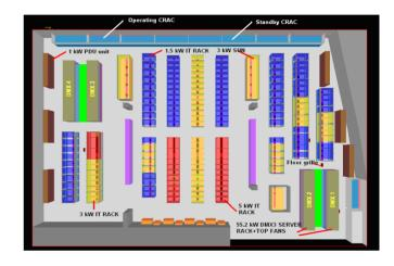
The spreadsheet is read by PHOENICS, enabling common data centre objects (i.e. CRACs, cabinets, floor / ceiling grilles) to be constructed automatically. This method allows rapid changes to be affected, such as scaling IT loads by changing a single value in the spreadsheet.
