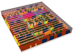
CHAM's PHOENICS CFD software, incorporates standard and product-specific objects for high- and low-density cabinets, racks, servers, PDU's, CRAC's and ACU's, as well as fans, diffusers and emergency fire suppression measures. Under-floor ventilation systems, cabling ducting, permeable and semi-permeable floor tiling are all taken into consideration, plus ceiling vents, grilles, extracts and recirculation systems.
