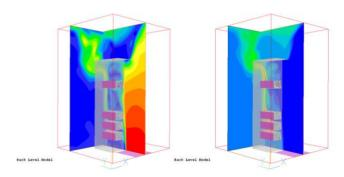
Ventilation and cooling systems for racks, blades and circuit board LED heat releases can be studied and exported to the larger scale model.
