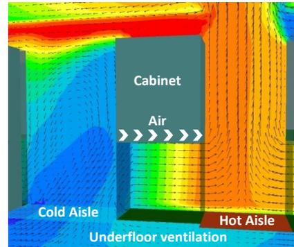
Results from the simulations show the air flows and temperatures into and out of the cabinets, indicating undesirable regions of recirculation from hot to cold aisles. PHOENICS also enables average and maximum inlet and outlet temperatures to all cabinets to be evaluated.
