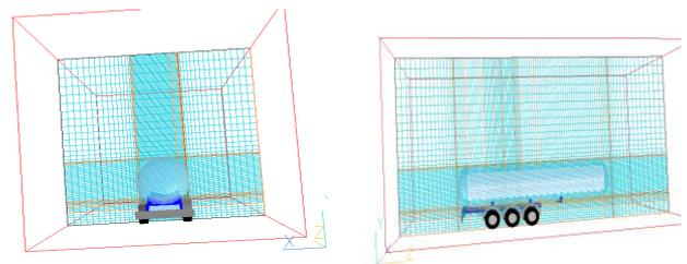
Comparison was made on the first half-hour of the experiment. In the computation, the fire was represented by a volume source term. The heat release rate of the tyre was deduced from measurements of heat fluxes.
