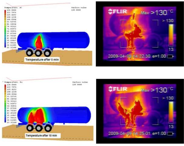
Comparison at 5 min and 10 min: computation and experiment (infra red camera)
