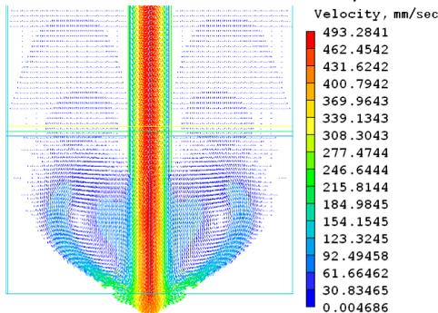
Fig.8 Velocity Vector of Liquid at the bottom part (0.2[sec])
