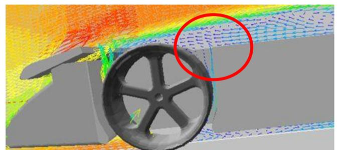
The above image shows the turbulence (circled) that the designers worked to eliminate through the design process.
