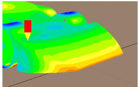
During the analysis process the designers looked at the coefficient of drag in the X, Y, and Z directions. The  $C_{dx}$  value held a heavier weight to the designers because this is the aerodynamic drag that is affecting the car. This gave the designers quantitative data which were compared to other designs. Also, with the use of the VR Viewer the designers could look at the velocity vectors. The designers looked for signs of turbulence which were easily viewable using the F1 VWT package.
