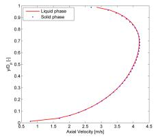
Figure 3. Axial velocity distribution along the vertical diameter (AB in Fig. 1) for the two phases. (7)
