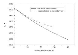
Fig. 6 The relationship between maximal temperature in a boiler and the flue gas recirculation ratio.
