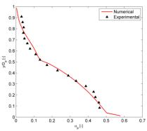
Figure 2. Solid volume fraction profile along the vertical diameter (AB in Fig. 1).
