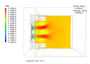
Fig. 5 The nitrogen oxide concentration field (recirculation ratio is 20%).
