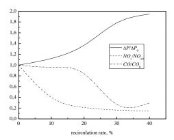
Fig. 8 The relationship between basic parameters of a DKVr 4/13 boiler and the flue gas recirculation ratio at the uniform recirculation.
