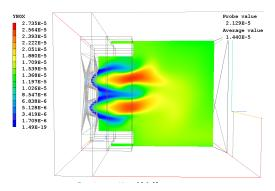
Fig. 3 – The nitric oxide concentration field.
