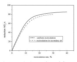
Fig. 7 The nitrogen oxide reduction as a function of a flue gas recirculation ratio and the way of its recirculation.
