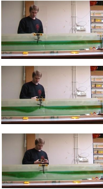
Figure 1 top to bottom (t=0s, 2s, 4s): development of the flow due to the paddle propelled carriage in a stratified tank (the top fresh water layer is dyed dark green). The carriage is moving from left to right.
