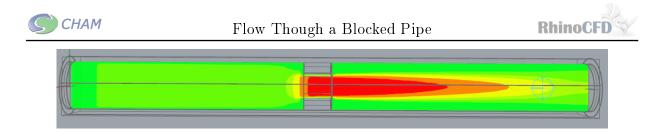
Figure 6: Velocity contour in Y plane
