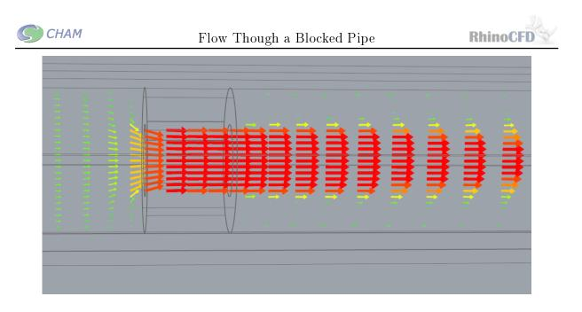
Figure 8: Velocity vectors in Y plane focused at blocked section
