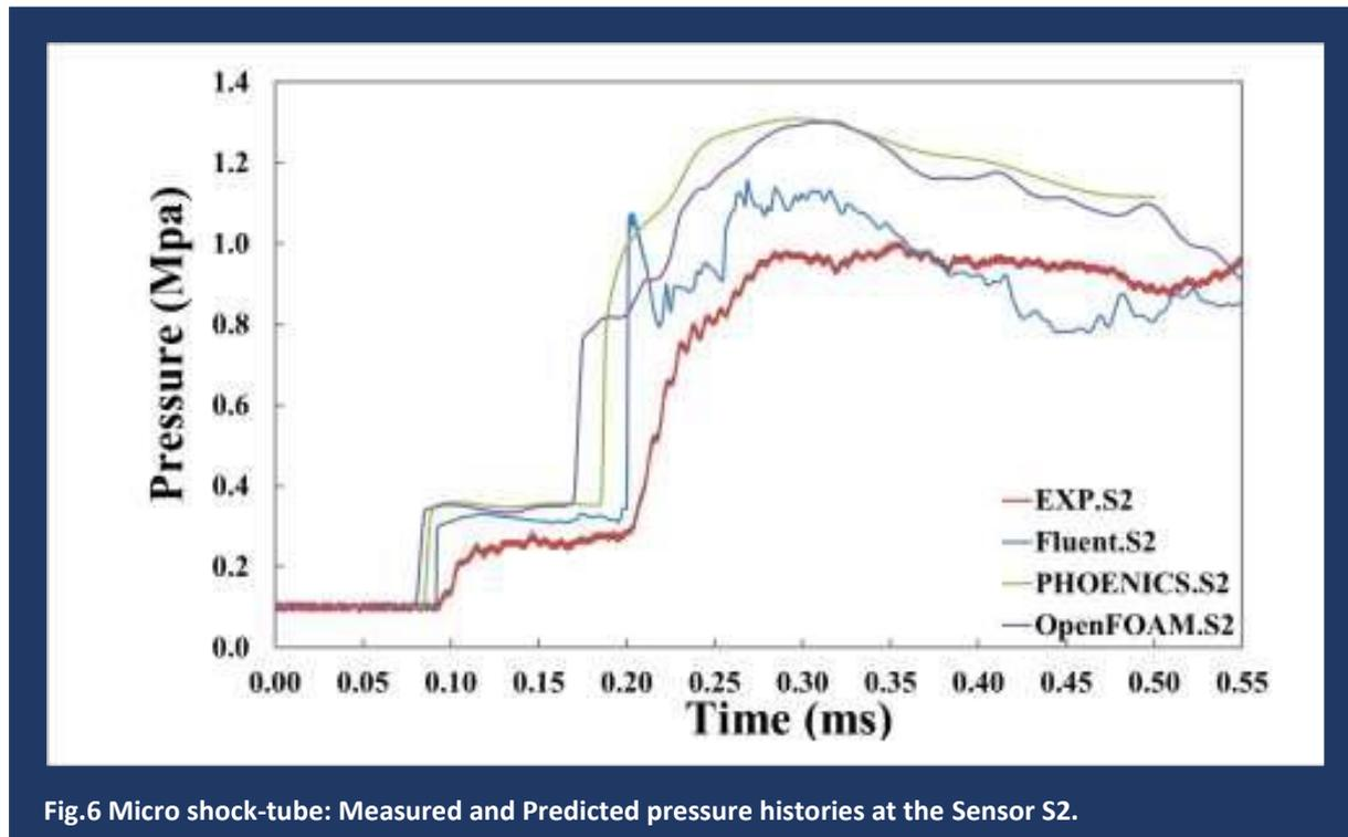
Fig.6 Micro shock-tube: Measured and Predicted pressure histories at the Sensor S2.
