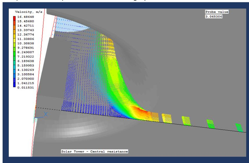
The cone is quite complicated internally but, for demonstration purposes, is represented simply as a blockage. [There is also a thermal storage reservoir underneath the tower complex to keep the turbine running overnight; this is ignored in the CFD model.]
