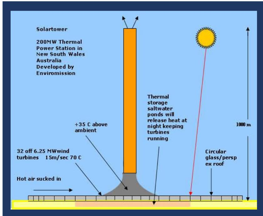
In this PHOENICS demonstration case, the grey cone sits at the centre of a large cylinder (about 6Km in diameter) representing Perspex covering, 3m high at the perimeter and 15m high at the base of the cone.
