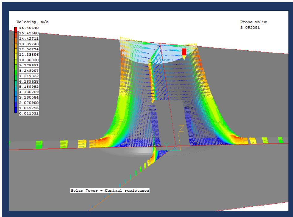
InForm is used to apply heat sources to hidden blockages, HEAT & HEAT2. The STORED variable MARK is set to 1 in all cells which are fluid and have a solid above them (ie on the next Z plane). Fluid cells are identified as having the property marker PRPS < 100, and solid cells as having PRPS > 99. Heat is applied to all cells with MARK=1.
