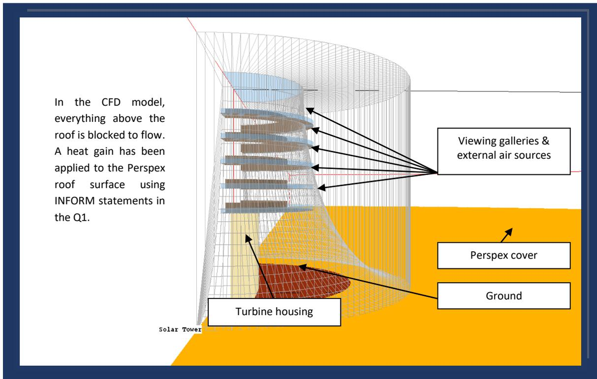
The above image shows the inside of the tower. There are 5 floors inside with viewing galleries, each with a wall at the inner end and an ANGLED-OUT at the outer edge. The ANGLED-OUTs intersect the blockage of the tower and provide fixed-pressure boundaries where they intersect.
