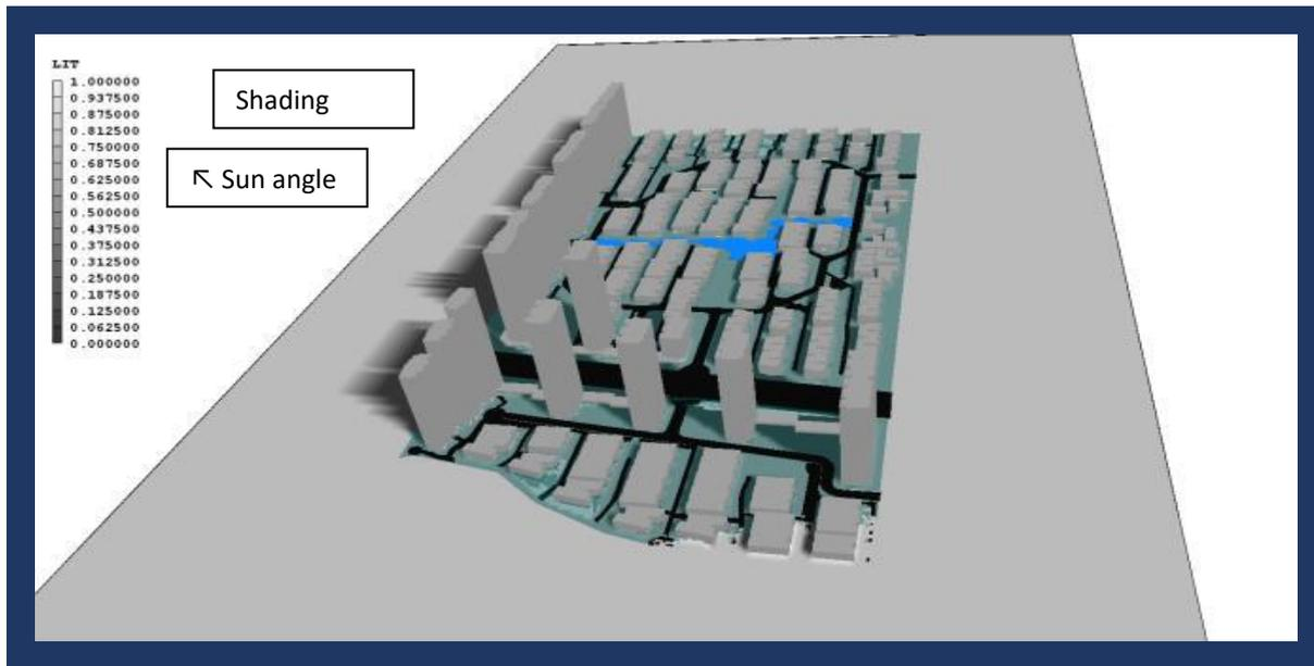
In this example, the ground surrounding the buildings, road, grass and river all have a Z depth of 2m. The ground temperature of 9°C is applied at the lower face of the ground. This represents the constant earth temperature underground.
