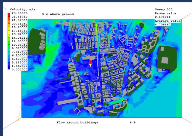
Wind velocity contours @ 5m above ground ↙ Wind
