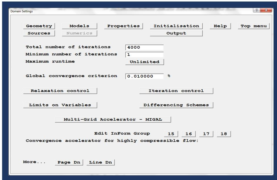
The default option for relaxation is *Automatic Convergence Control* (CONWIZ): On. This is a convergence wizard that automatically sets the relaxation parameters to try to ensure convergence. If it is switched off, experienced users can set parameters manually, which can lead to faster run times using less conservative relaxation values.
