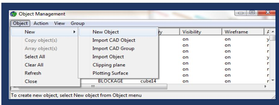
Select *New Object* and set object type to *Sun* object. Then, by clicking attributes, the following panel appears, for which relevant data can be specified.
