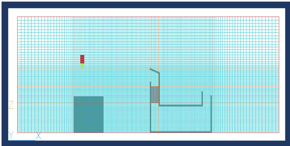
In certain regions it might be beneficial to crush the mesh using non-uniform spacing to reduce the overall cell count. Both *Power* and *Geometric Progression* distributions are available, with power/ratio settings  $<-1$  for diminishing and  $>1$  for increasing mesh spacing.
