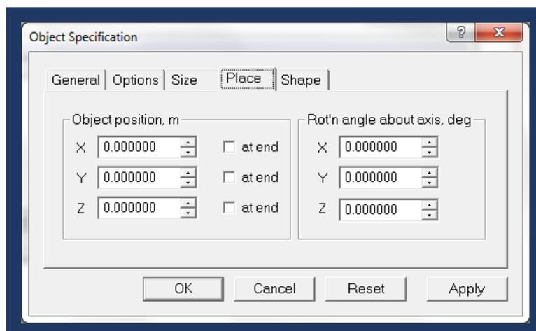
Likewise, an *Opening* (or outlet) object must be added on the far right of the domain. This is a pressure boundary, with flow through it governed by the difference in pressure inside the domain and the external reference pressure (normally set to ambient pressure). The position of this outlet is set to X "at end" or at 30m.
