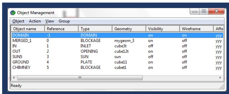
With the geometry set up, the domain settings are applied.
