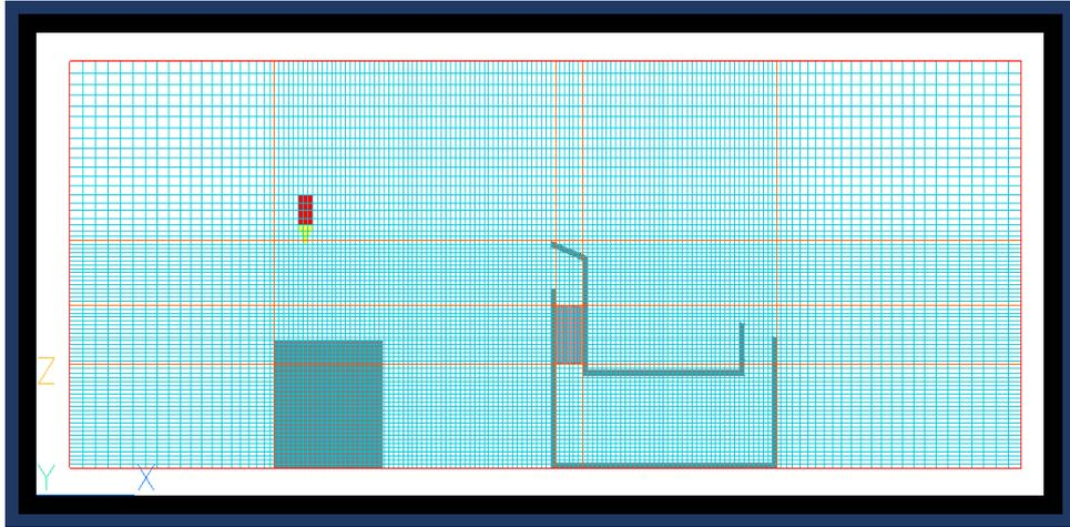
Clicking the mesh button on the control panel displays the mesh overlaid on the domain. Each of the regions (created by objects affecting the grid and denoted by orange lines on the mesh display) can be modified individually by clicking them and changing the desired parameter on the *Grid Mesh Settings* panel.
