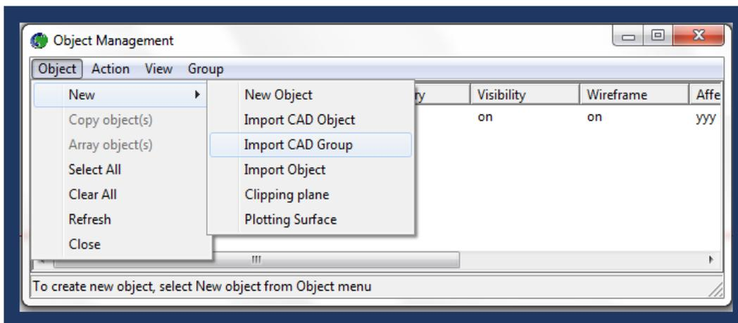
Once it is selected, the following screen will appear. We have the option to scale the CAD object in question, which can be useful if units used for the CAD file are not in metres (PHOENICS default is to use SI units.)
