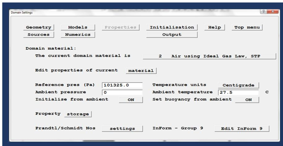
Buoyancy is set in the *Sources* panel. This option is set automatically to the *Density Difference* method if *FLAIR* is used.
