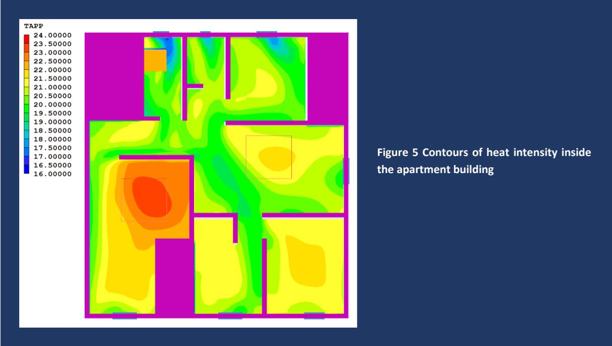
Figure 5 Contours of heat intensity inside the apartment building
