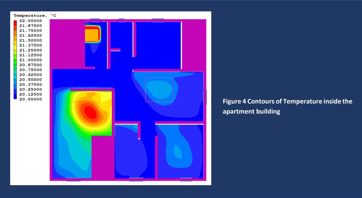
Figure 4 Contours of Temperature inside the apartment building
