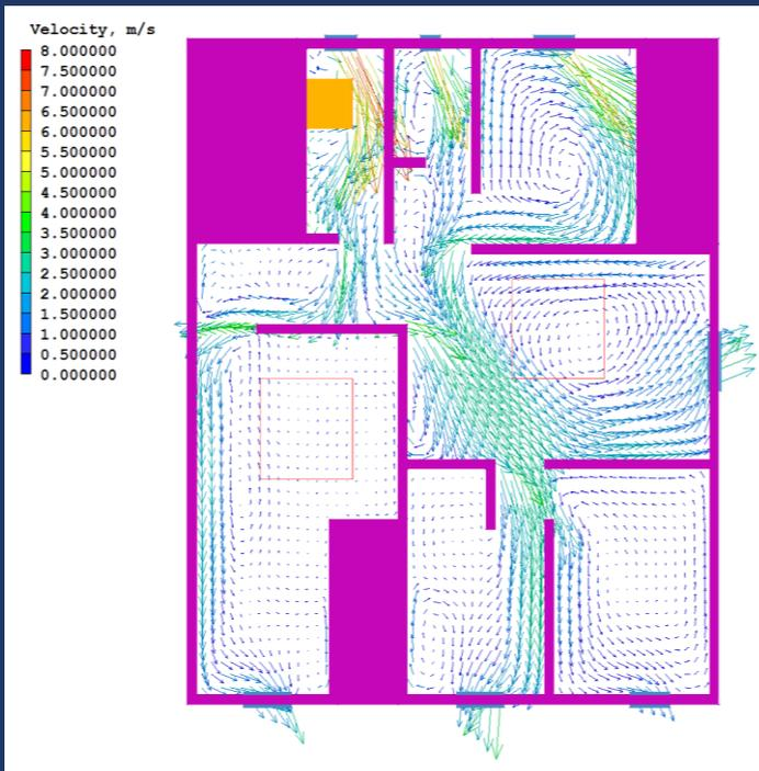
Figure 3 Vectors coloured by velocity at 1.5m above the apartment floor
