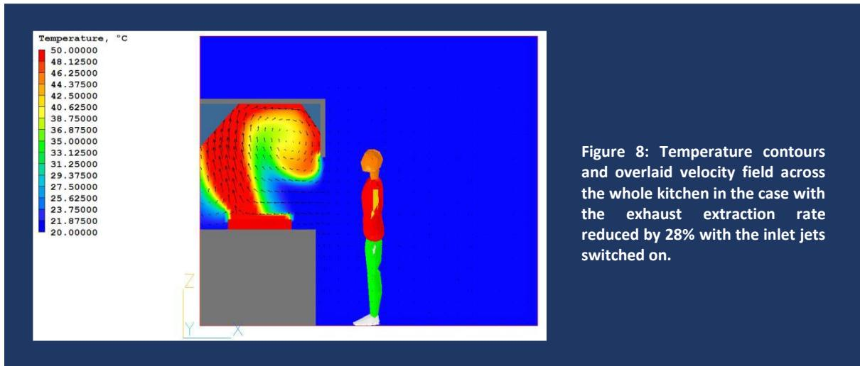
**Figure 8:** Temperature contours and overlaid velocity field across the whole kitchen in the case with the exhaust extraction rate reduced by 28% with the inlet jets switched on.
