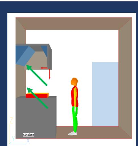
**Figure 1: Geometry of the kitchen and KVI unit located above the hob (shown red). The inlet locations are marked by a red arrow showing the direction of air injection. The angled outlet is the blue wedge on the left of the hood and is indicated by a green arrow.**
