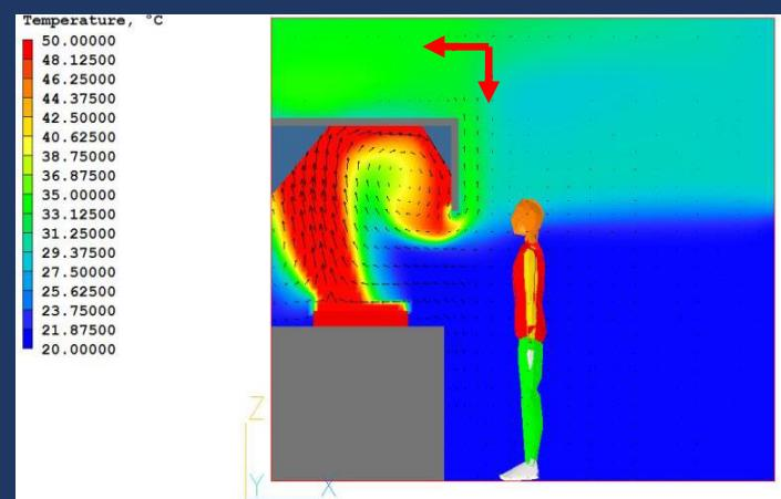
Figure 7: Temperature contours and overlaid velocity field across the kitchen in the case with the exhaust extraction rate reduced by 20% (as in Figure 4) with the inlet jets switched on.
