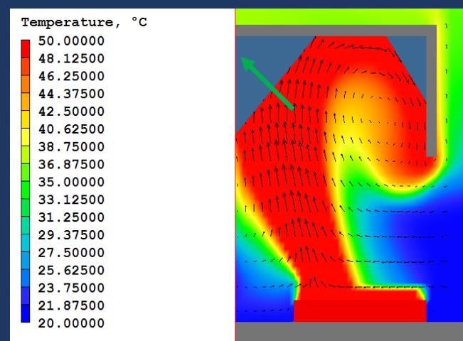
**Figure 4:** Temperature contours and overlaid velocity field in a case with 20% exhaust reduction and the KVI inlet jets switched off.
