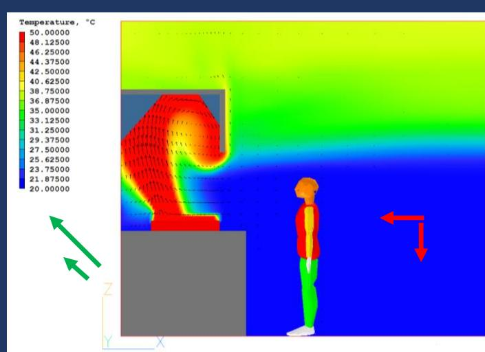
Figure 5: Temperature contours and velocity field across the whole kitchen in the case with 20% exhaust reduction and the KVI inlet jets switched off.
