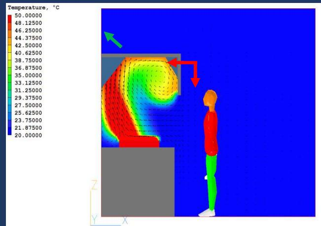
**Figure 3:** Temperature contours and overlaid velocity field across the whole kitchen in a case where KVI inlet jets are switched on.
