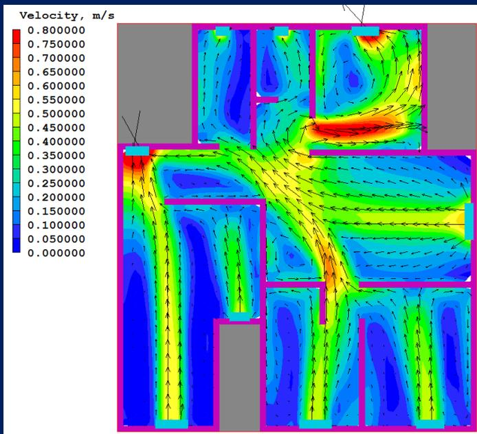
Figure 3 Velocity contours and vectors at  $z=1.45\text{m}$
