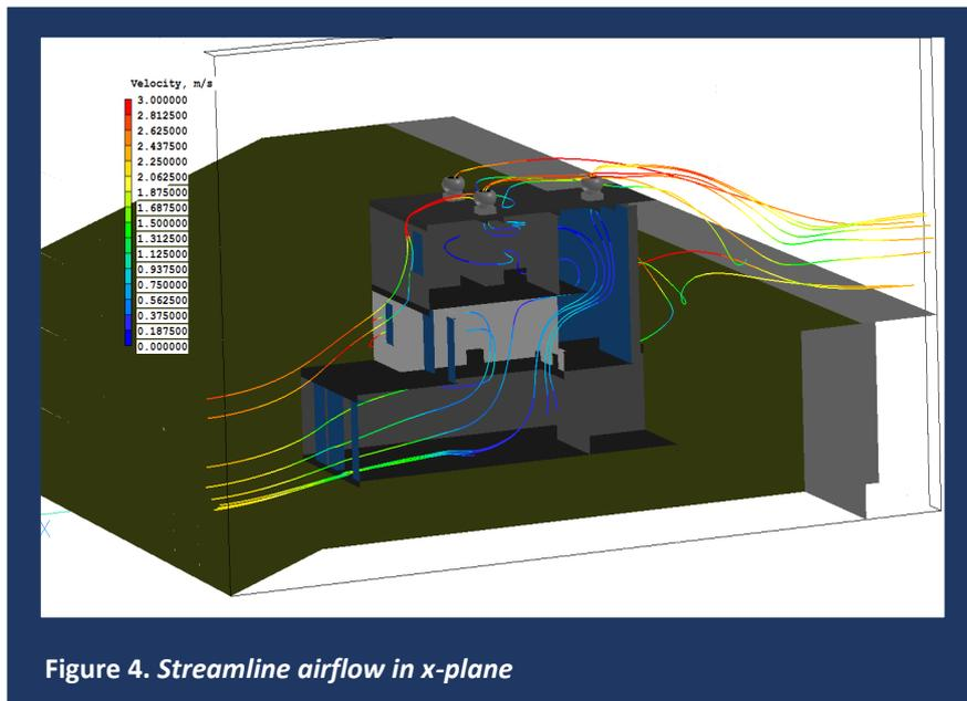
The CFD model can be used to ascertain, quickly and inexpensively, whether more-restricted openings through the lower region would balance flow on each floor to the required degree, or if other remedial action might be needed.
