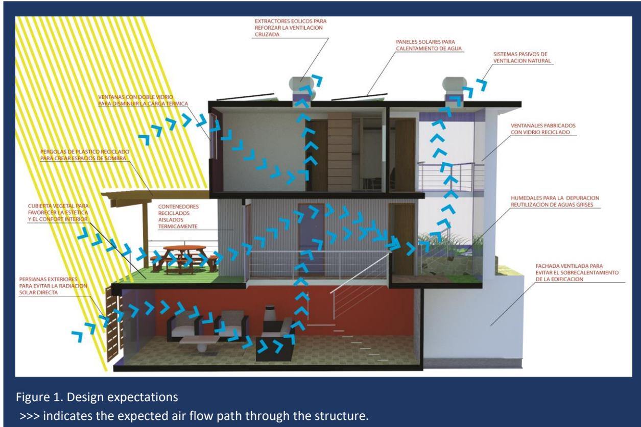
In this demonstration, PHOENICS/FLAIR is used to analyse the natural ventilation of a concept home, comparing it to initial expectations. The building is a private house, to which full recycling and bioclimatic concepts have been applied. The building consists of re-cycled shipping containers and was designed by ASOLBA Ingeniería & Arquitectura, a firm of sustainable design and energy efficiency engineers located in Guayaquil, Ecuador and Barcelona, Spain.
