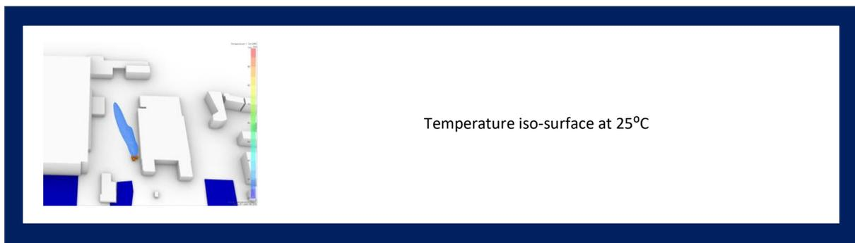
The results showed that, for the scenario considered, the hot air exhausted from the load banks has little effect on their immediate surroundings, being diluted rapidly by the on-shore wind and rising rapidly above head height due to buoyancy. Similar iso-surfaces of the hot air, plotted at the more-critical temperature of 50°C, indicate even smaller impact.
