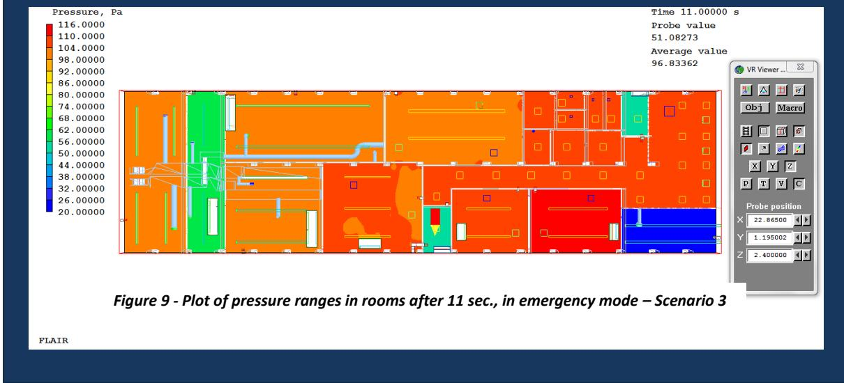
**Figure 9 - Plot of pressure ranges in rooms after 11 sec., in emergency mode – Scenario 3**
