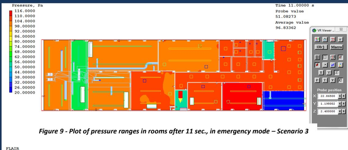
The analysis of each scenario simulated showed that the pressure in the rooms attained the required level very quickly and no case exceeded 9 seconds. The rate of increase in pressure can also be calculated using mathematical formulas, not only via CFD modelling.
