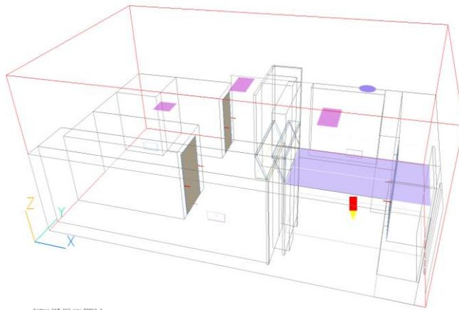
A 3D CFD model was built from 2D CAD plan drawings, provided by the client. The dimensions of the domain containing the LAF unit cleanroom were  $\sim 11.5\text{m} \times 7\text{m} \times 5\text{m}$ . Figure 1 shows a perspective view and a plan view of the room. Walls, floor and ceilings that obstruct the view have been hidden.
