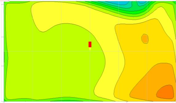
Figure 3 – Zoomed view of velocity at workbench directly beneath LAF unit
