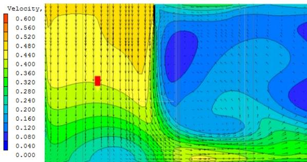
Figure 4 – Side On view showing velocity on a section across the middle of the LAF unit
