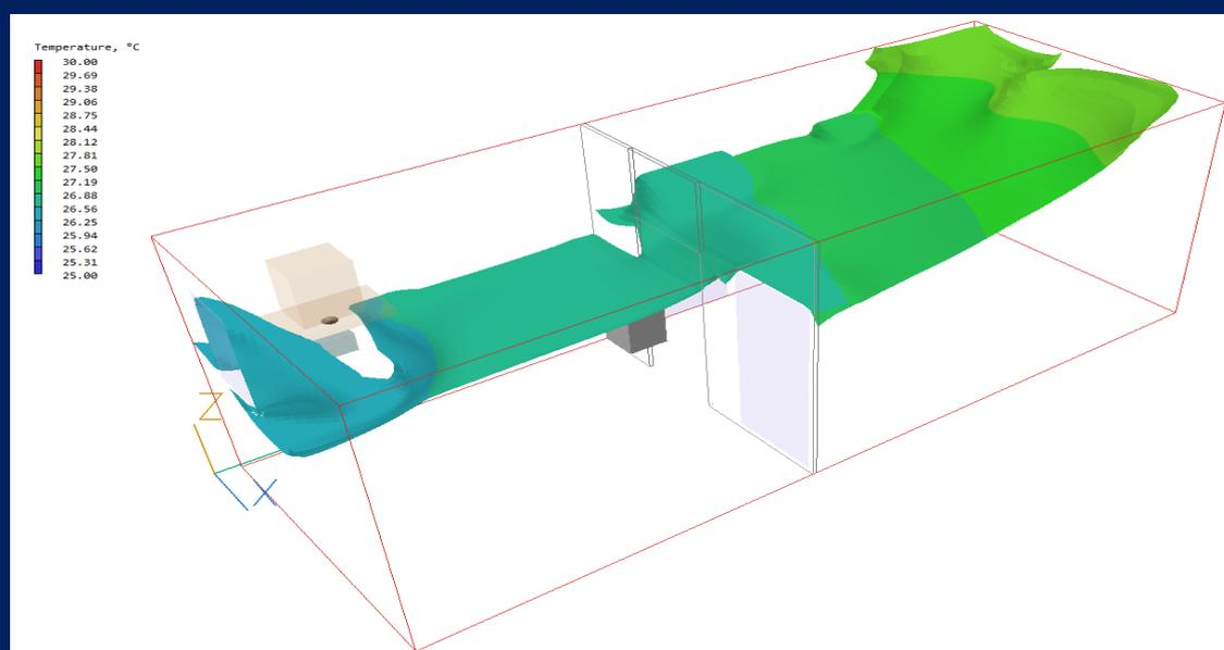
Figure 3: Iso-surface plot of PM2.5 concentration ( $60 \mu\text{g}/\text{m}^3$ ) coloured by temperature.
