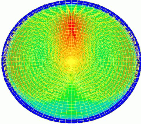
*Velocity vectors & temperature contours in cooled tubes influenced by gravity acting in the vertical direction.*
