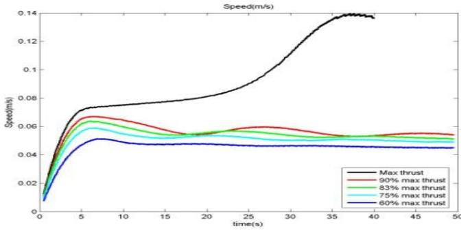
**Figure 1.** Body speeds at various thrust values as a function of time centerline and tank wall at 40s from start for the case at 60% thrust changing to 100% thrust after 15s are shown in figure 3. Figure 4 gives a clearer idea of the waves created using vertical velocity contours and flow vectors. This figure clearly shows mode 1 internal waves travelling both behind and in advance of the moving body (the position of which can be identified by the area of parallel surface velocity vectors).
