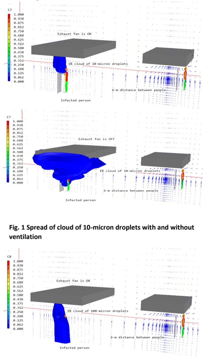
**Fig. 1 Spread of cloud of 10-micron droplets with and without ventilation**
