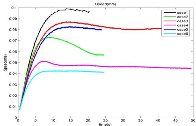
**Figure 5.** Body speed versus time for 6 simulations. Cases 1 and 2 have body draft of 0.015m with case 1 being the non-stratified equivalent to case 2. Cases 3 and 4 have body draft of 0.030m with case 3 being the non-stratified equivalent to case 4. Cases 5 and 6 have body draft of 0.040m with case 5 being the non-stratified equivalent to case 6.
