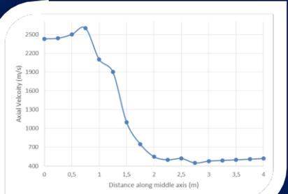
b) Axial centerline velocity of jet exhaust
