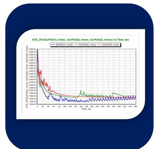
Different temperatures were calculated at the top boundary condition (20, 60 and 40 Celsius). Image analysis demonstrated that water surface evaporation can have stochastic characteristics which depend on the flow structure changing.
