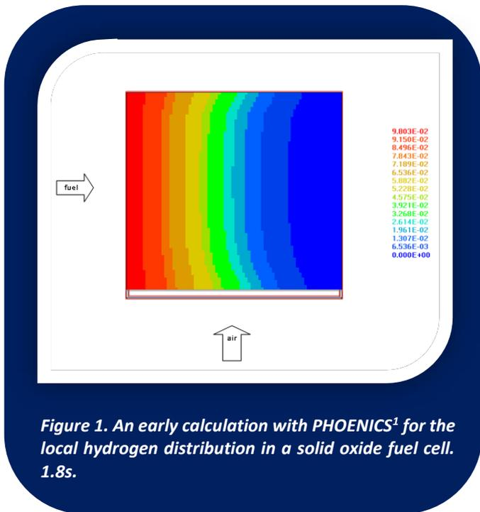
Figure 1. An early calculation with PHOENICS<sup>1</sup> for the local hydrogen distribution in a solid oxide fuel cell. 1.8s.
