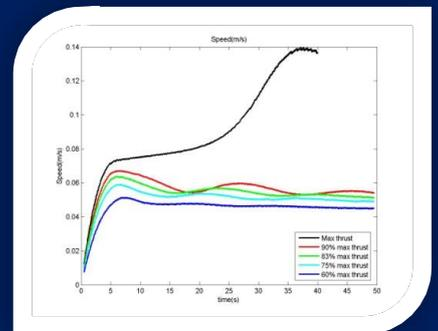
*Figure 7. Propelled body speeds at various thrust values as a function of time.*
