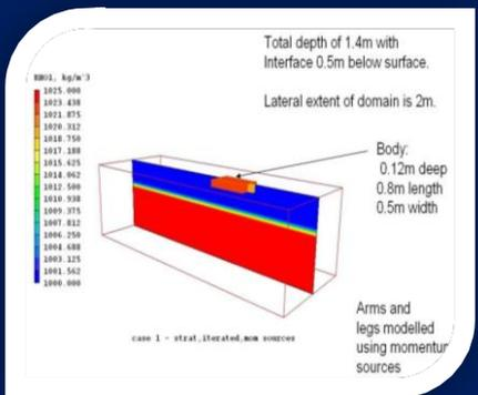
Figure 2. Representation of a swimmer swimming in stratified water with moving arms and legs.
