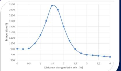
c) Axial temperature starting from jet exhaust
