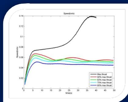
*Figure 7. Propelled body speeds at various thrust values as a function of time.*
