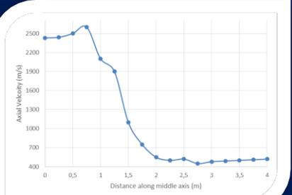
b) Axial centerline velocity of jet exhaust
