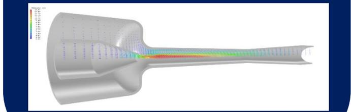
**Figure 5 – Velocity vectors coloured by velocity magnitude.**
