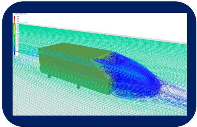
The slant on the Ahmed used in our case study had an inclination of 25 degrees which from the experimental data corresponds to a Cd of 0.342 (Meile W. B., 2011).
