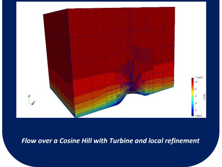
Flow over a Cosine Hill with Turbine and local refinement
