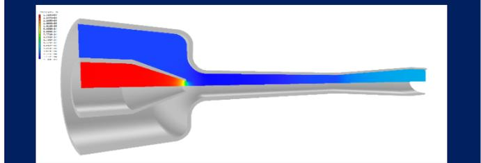
**Figure 4 – Surface contour of Total Pressure relative to an ambient pressure of 101325 Pa.**
