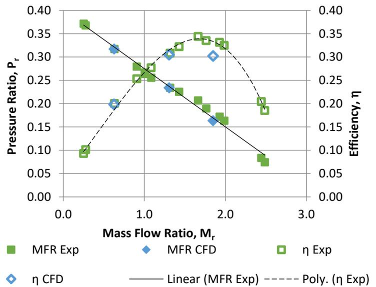
**Figure 2 – Mass Flow Ratios (MFR) against Pressure Ratios and Efficiency. Experimental data represented by green squares with a linear best-fit line (-) for MFR and a third order polynomial best-fit dashed line (- -) for Efficiency. PHOENICS CFD derived data is represented by blue diamonds.**
