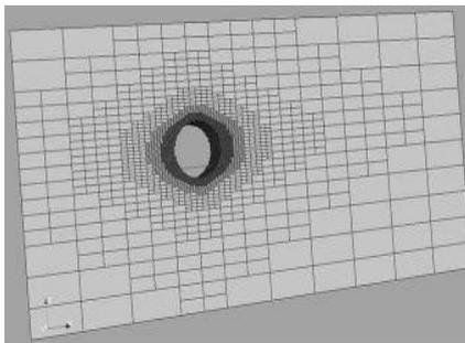
As can now be seen, USP cells are always rectangular, and of uniform aspect ratio. Although vendors of other CFD packages often employ unstructured grids in which the cells are of arbitrary rectangular shape, CHAM sees no significant advantage in so doing.
