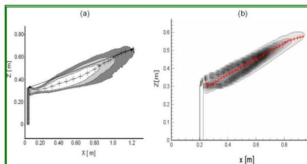
Figure 1. Mean flame trajectory for a cross flow velocity  $V_\infty$  of 2.0 m/s, ( $V_j/V_\infty=0.5$ ), a) Experimental data (Majeski, et al. 1999) and b) Numerical results (flame borders are defined by means of heat radiation contours).  $V_j$  is the propane discharge velocity and  $V_\infty$  corresponds to the cross flow velocity.
