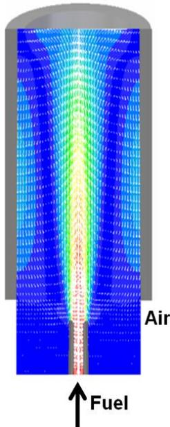
Figure 4. Flow field predictions of the fuel-air mixture.
