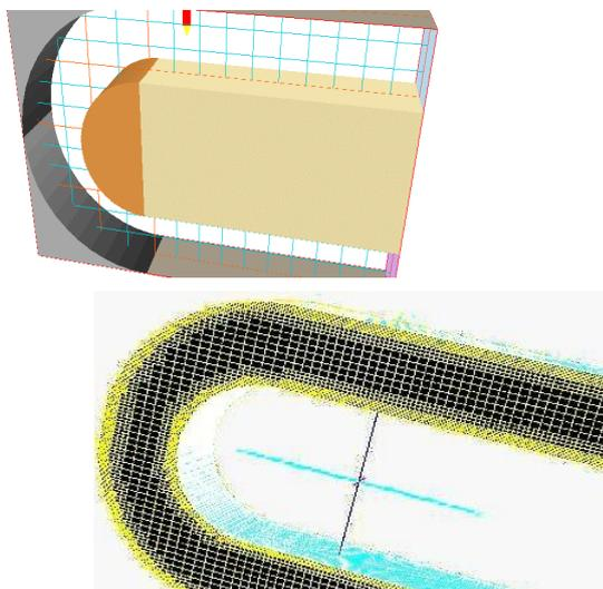
Next is shown the near-surface grid refinement of a three-dimensional example, with several differently-shaped objects.
