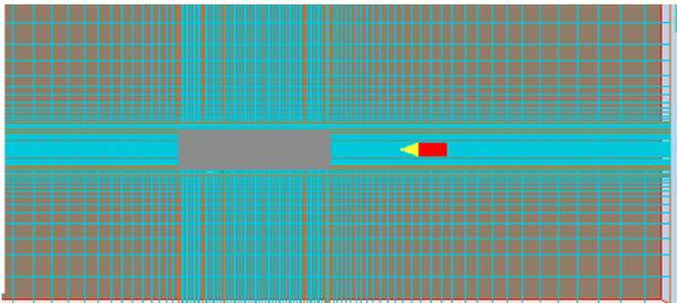
USP removes this necessity, as is shown below: the fine-grid region hugs the surface of the central body, which is where it is needed for procuring accuracy; farther from the body the cells are larger, and also of acceptable aspect ratio.
