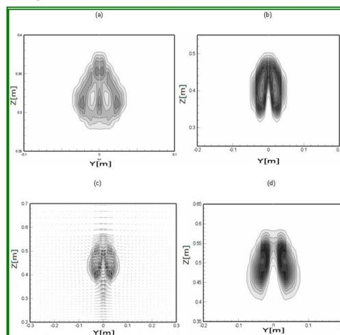
Figure 2. Mean shape for  $V_j/V_\infty=0.5$  at four different downstream locations of the stack: a)  $x/D=3.5$ , b)  $x/D=17$ , c)  $x/D=21$  y d)  $x/D=26$ . Flame borders are defined by means of heat radiation contours.  $V_j$  is the propane discharge velocity,  $V_\infty$  corresponds to the cross flow velocity and  $D$  is the diameter of the stack.
