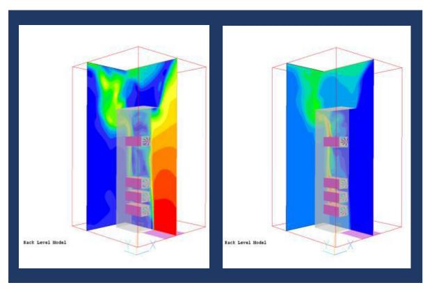
Ventilation and cooling systems for racks, blades and circuit board LED heat releases can be studied and exported to the larger scale model. From macro-scale to micro-scale data centre problems, PHOENICS/FLAIR offers a solution.
