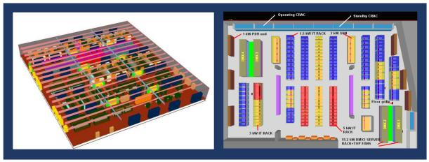
The spreadsheet is read by PHOENICS, enabling common data centre objects (ie CRACs, cabinets, floor / ceiling grilles) to be constructed automatically. This method allows rapid changes to be effected, such as scaling IT loads, by changing a single value in the spreadsheet.
