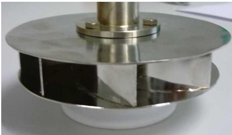
Picture of a typical "induced-draft rotor" used for foam separation
