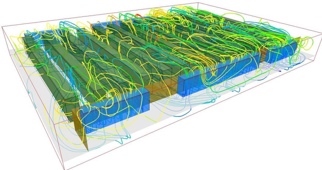
Figure 2 Streamlines through cabinets and return paths to CRAC units (blue)
