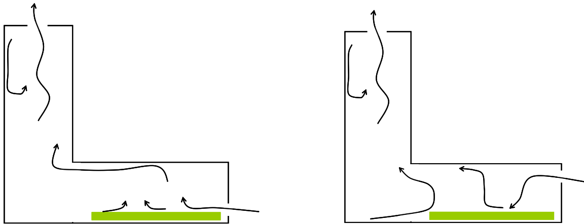
Figure 48. Airflow Patterns for Single Heated Zone Case from Airflow Visualization in the Model: a) Lower Windows, b) Upper Windows
