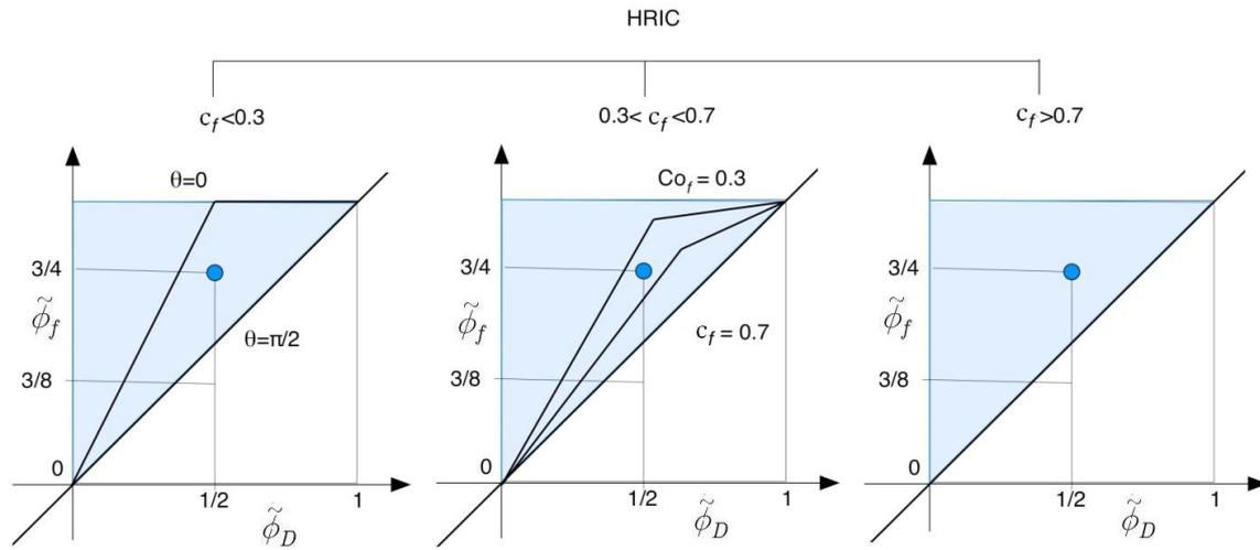
Figure 4: NVD for the HRIC scheme at different Courant numbers.
