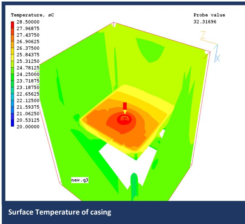
The casing temperature rose by around 5°C, and the bracket supporting the LEDs rose by 8-9°C.
