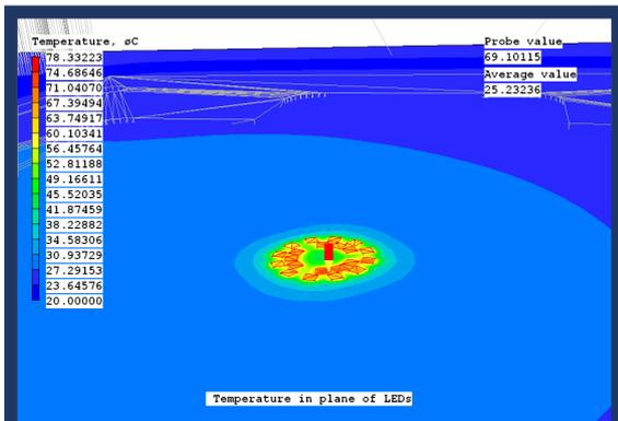
Temperature in plane of LEDs
