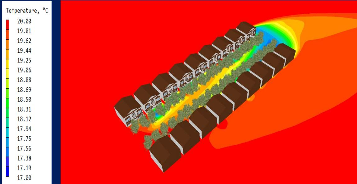
Figure 5: Contour plot of temperature at pedestrian level showing up to 3 °C of cooling towards the leeward end of the street. Scale: Red – 20 °C; Blue – 17 °C
