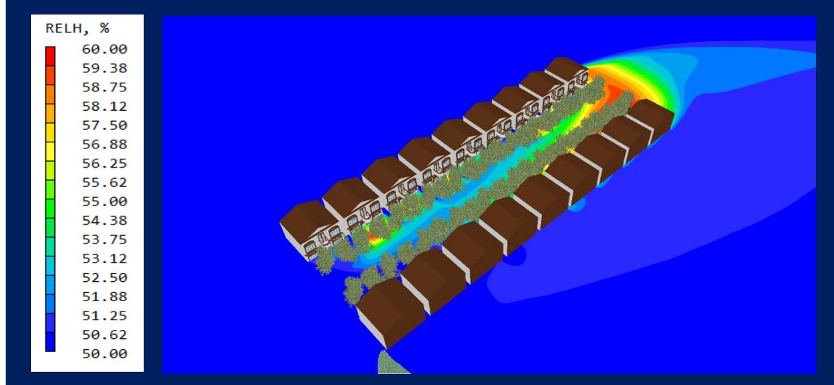
Figure 4: Contour plot of relative humidity at pedestrian level showing up to an increase of 10% humidity towards the leeward end of the street. Scale: Red – 60 %; Blue – 50 %
