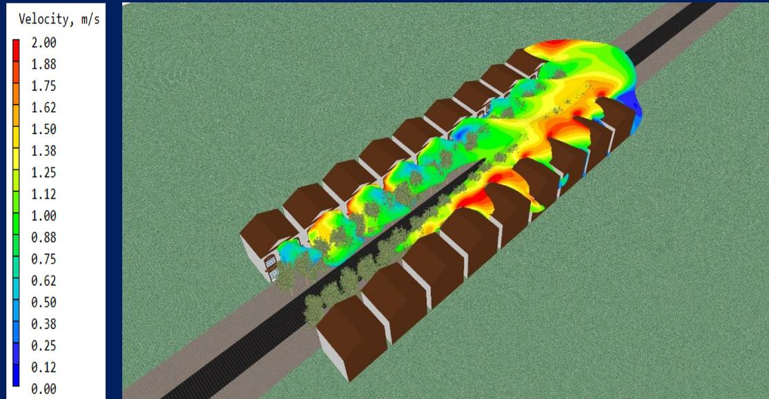
Figure 7: Iso-surface plot of temperature at 19 °C, coloured by velocity, demonstrating that the majority of the street experiences at least 1 °C of cooling due to evapotranspiration.
