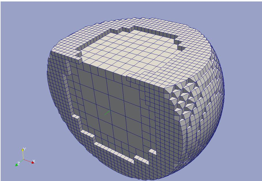
**Fig. 4.3** The sphere mesh
