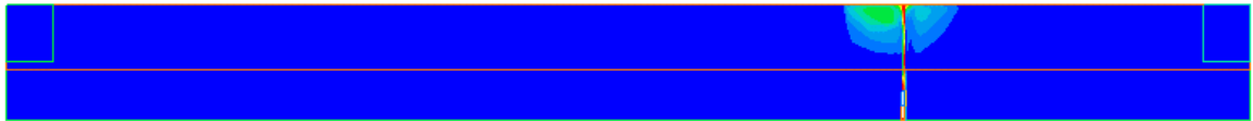
Figure 19 Temperature contours at a section through the centre of the tunnel at 1 minute
