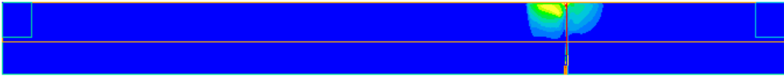
Figure 31 Temperature contours at a section through the centre of the tunnel at 1 minute
