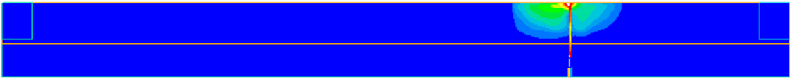
Figure 37 Temperature contours at a section through the centre of the tunnel at 1 minute
