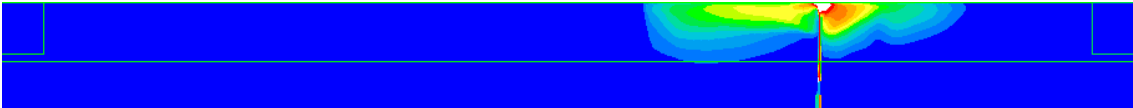
Figure 43 Temperature contours at a section through the centre of the tunnel at 1 minute
