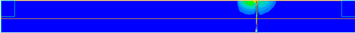
Figure 25 Temperature contours at a section through the centre of the tunnel at 1 minute
