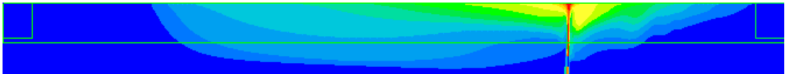
Figure 57 Temperature contours at a section through the centre of the tunnel at 5 minutes
