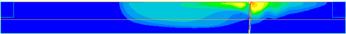
Figure 15 Temperature contours at a section through the centre of the tunnel at 5 minutes
