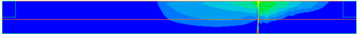
Figure 21 Temperature contours at a section through the centre of the tunnel at 5 minutes
