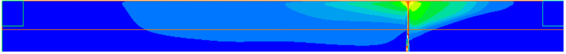
Figure 23 Temperature contours at a section through the centre of the tunnel at 10 minutes
