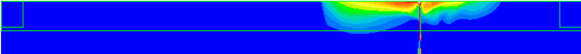
Figure 55 Temperature contours at a section through the centre of the tunnel at 1 minute
