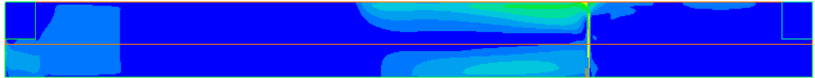
Figure 22 Velocity contours at a section through the centre of the tunnel at 5 minutes
