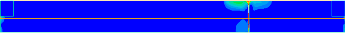
Figure 38 Velocity contours at a section through the centre of the tunnel at 1 minute
